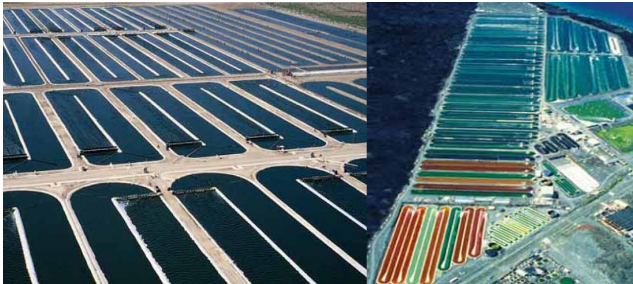
Fig. 2.B.1. Commercial microalgae production in open raceway paddle-wheel mixed ponds. A. Left; Earthrise Nutritionals, LLC, California. Production of Spirulina , Ponds ~ 1 acre. B. Right: Cyanotech Co., Hawaii, producing Haematococcus pluvialis (red ponds) and Spirulina .
