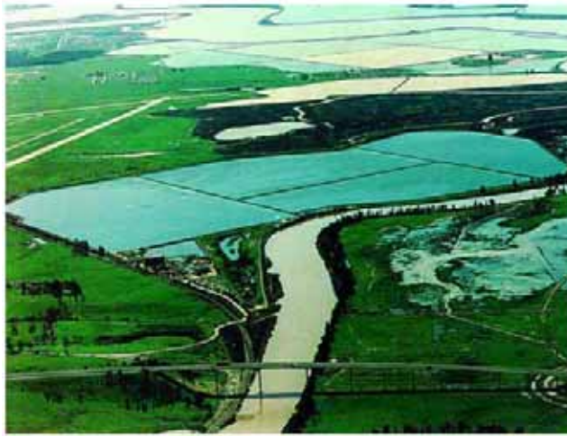
Figure 2.A.1. Oxidation Pond for Wastewater Treatment (Napa, California, total ~300 acres) Note: ponds on top are salt evaporation ponds.
