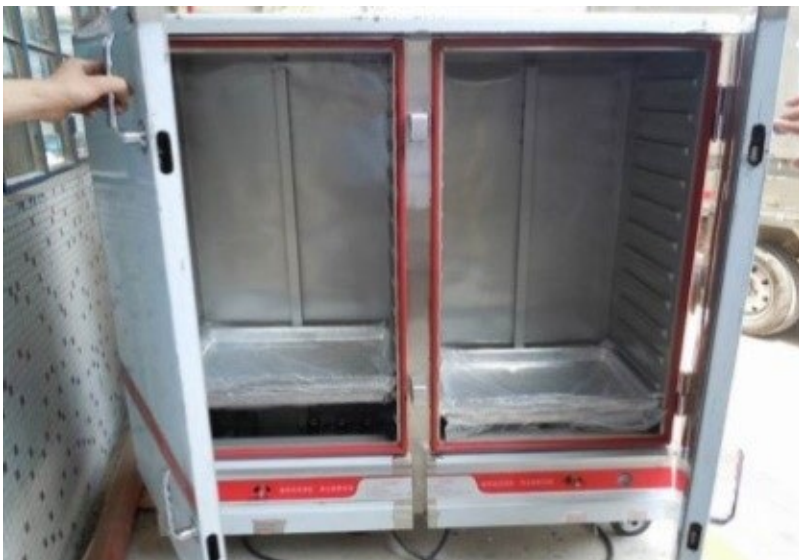
Figure 2-8 Methanol Steam Cabinet
