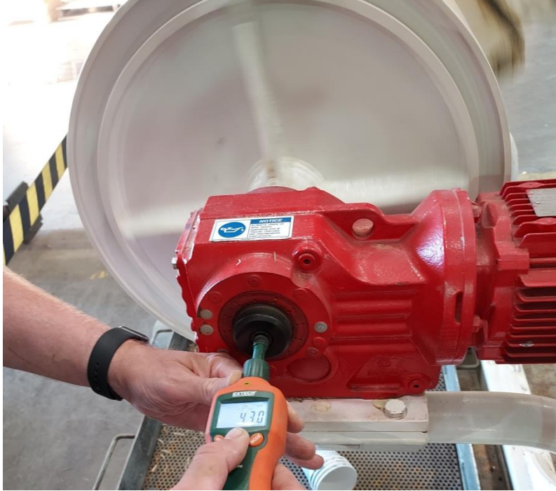
Figure 3-17 Checking RPM on Shaft Mounted Direct Drive Electric Motor
