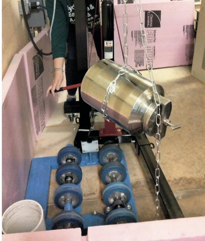
Figure 3-16 Experimental Off-Loading 5 Liter MSE Vessel from Morse Roller Rig
