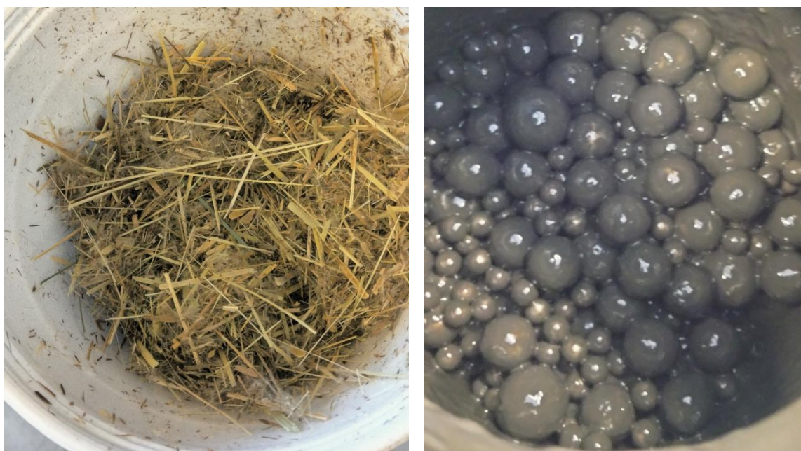
Figure 1-8 Before and After Switchgrass Ball Milling & Enzyme Hydrolysis
