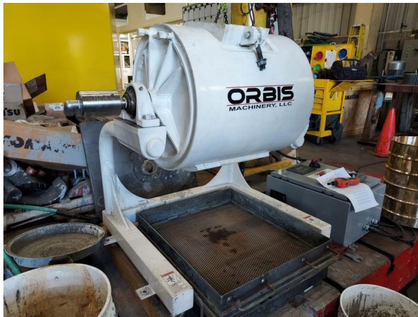
Figure 1-1 Commercial Scale Ball Mill used for process development.
